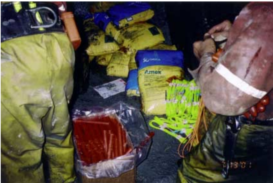
Plate 4. Explosive Product and Non-Electric Detonators used for Blasting Operations.
