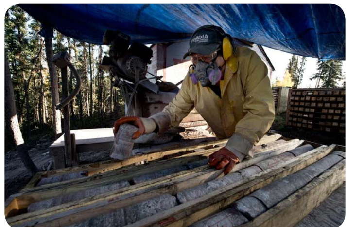
Ricky Drygeese cutting a small slice of core sample to be shipped to Vancouver for further examination.
