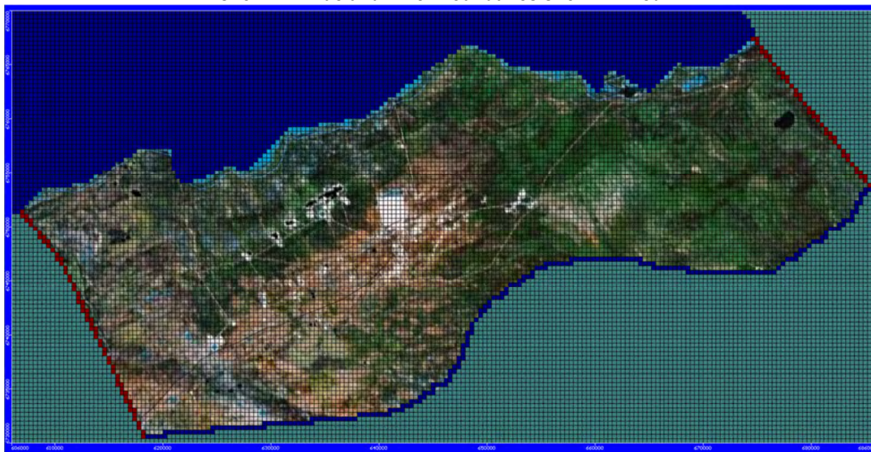
Figure 6: Pine Point area Groundwater Flow Model Constant Head Boundaries shown in Blue and River Boundaries shown in Red
