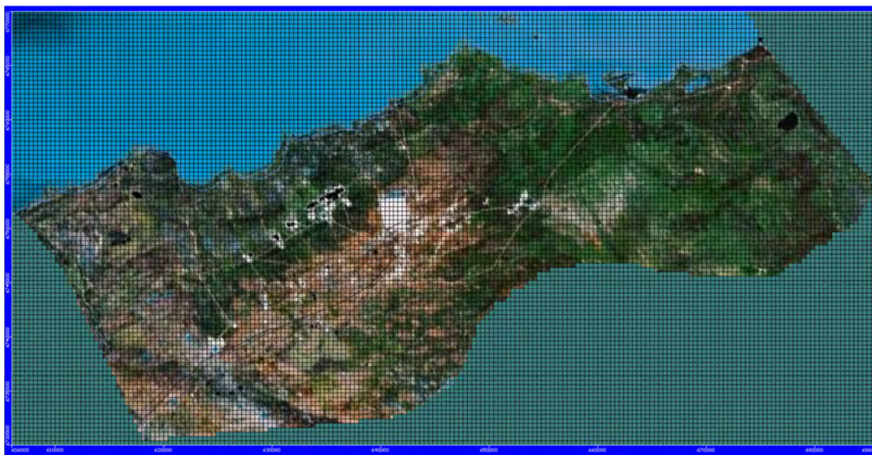
Figure 5: Pine Point area Groundwater Flow Model Domain and Discretization
