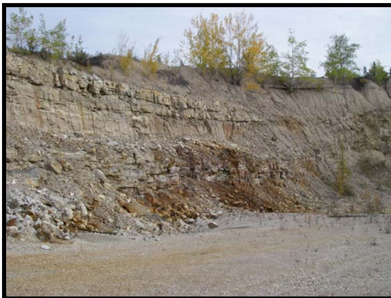
Photo 8 – View showing till with minimal organics overlying bedrock.
