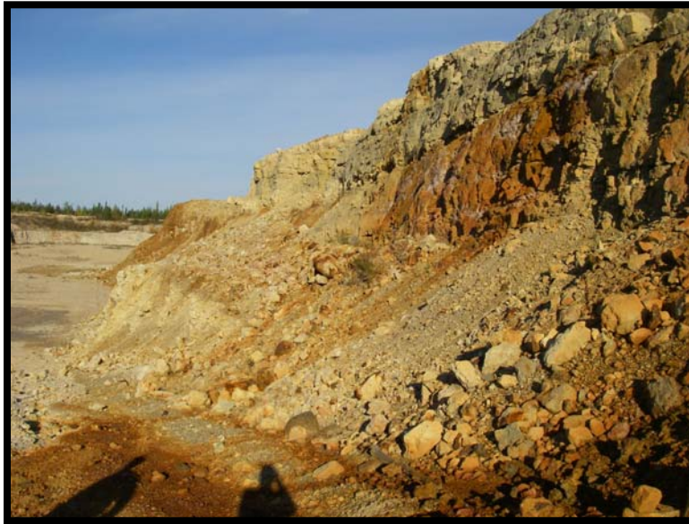
Photo 17 – View showing N-33 Pit wall seepage from bedding plane.
