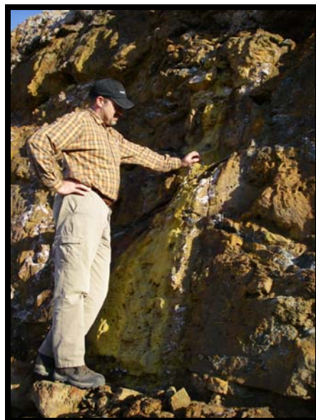
Photo 18 – N-33 Pit wall seepage discharge.
