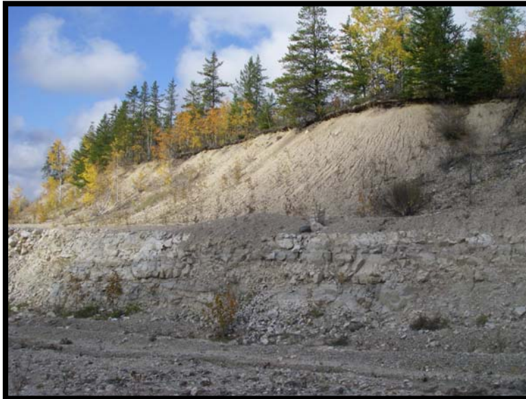
Photo 9 – View showing till overburden with rilling (small erosion gullies).
