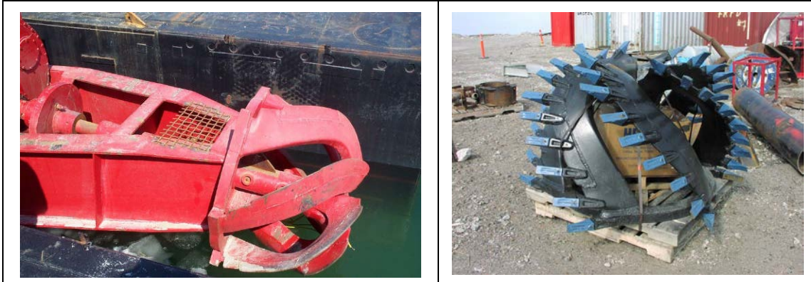
Figure 4-1. Cutter head used for A154 dredging (left), and toothed cutter head used for A418 dredging (right). Photos from NKSL (2003 and 2007a, respectively).
