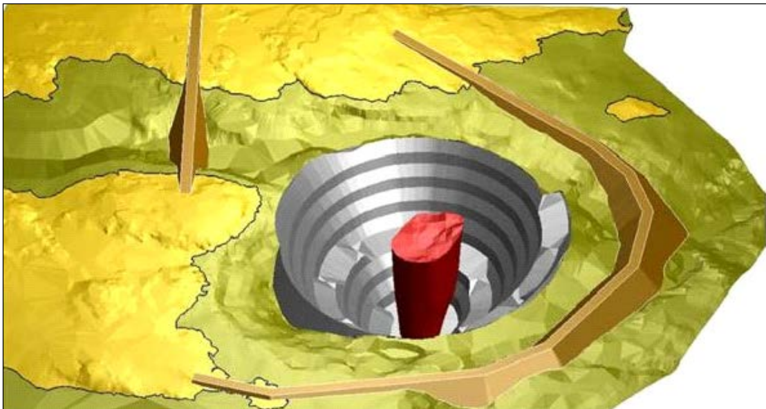
Figure 1-2. 1999 feasibility study A21 dike alignment (isometric).
