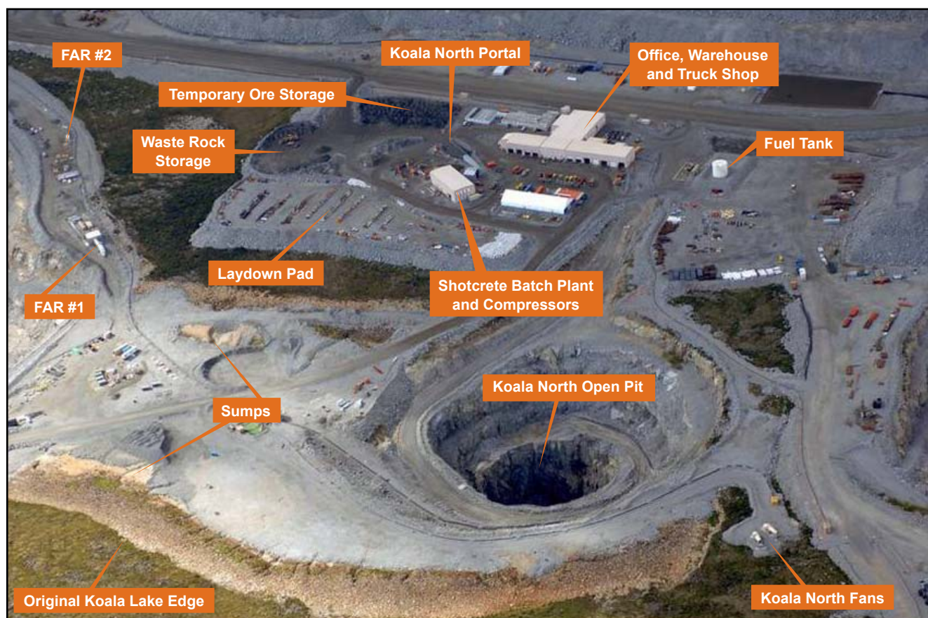
Aerial view showing above-ground support facilities and portal to underground mining operations.
