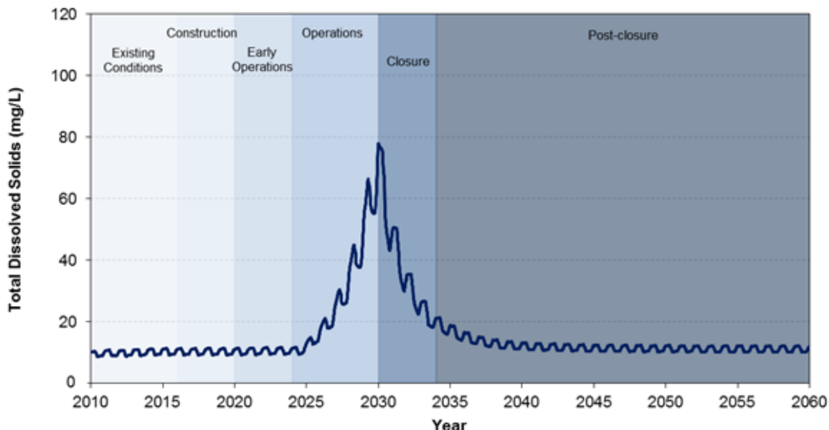
Figure 9.4-6 TDS Concentrations Predicted to Occur in the Main Basin of Lac du Sauvage
