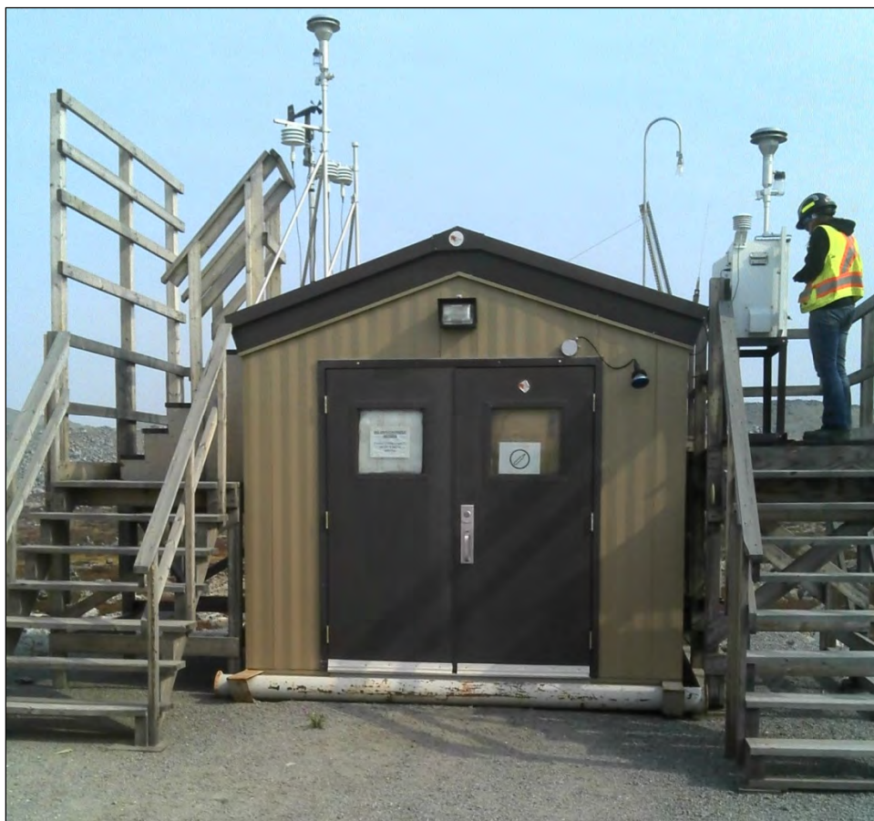
Plate 2.3-3. The continuous air monitoring (CAM) station. Houses internal equipment to continuously measure SO 2 , NO 2 , NO, NO x , TSP and PM 2.5 . The CAMB Partisol sampler configured to sample PM 2.5 is attached to the right of building, August 2014.
