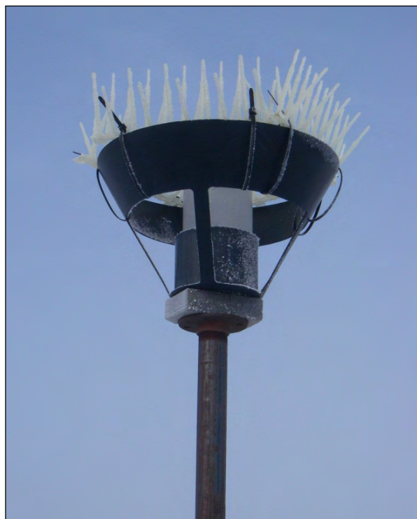
Plate 2.5-2. Close-up view of a dustfall collector during a non-sampling month, May 2011.
