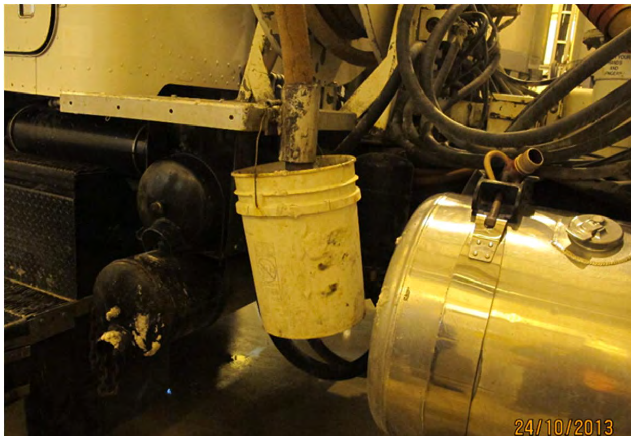
Figure 4-2: Bucket Used to Catch any Emulsion that May Drip from the Hose.
