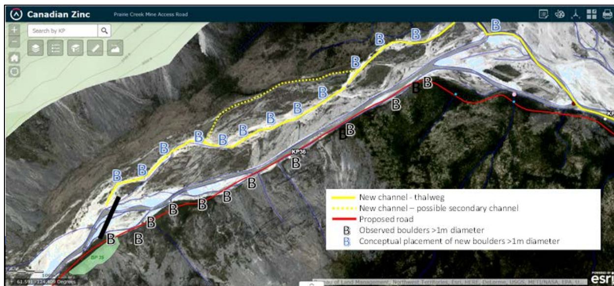
Figure 1 Sundog Creek, conceptual placement of boulders in new channel to approximate habitat lost in original channel.
