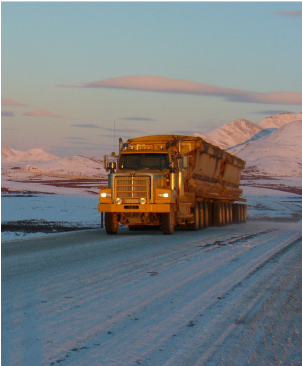
Figure 15 Concentrate truck on haulage road in the Arctic and in the shop for maintenance. Notice the tarp roof and the spansets securing it. In this particular case concentrate is loaded in bulk. The road is mostly flat with very moderate cross slopes.
