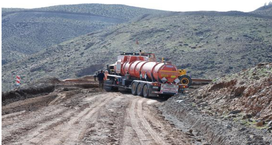
Figure 22 Trailer tanker lost adherence and started slipping back on access road. Grader came in to help as it was performing maintenance. Road was blocked for more than one hour. Note the road width (approx. 8 m). Left side is indicated by a red/white vertical signal, a small protective berm is present on the shoulders, both sides.
