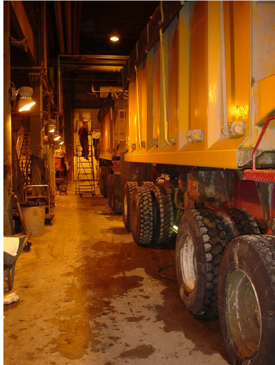
Figure 15 Concentrate truck on haulage road in the Arctic and in the shop for maintenance. Notice the tarp roof and the spansets securing it. In this particular case concentrate is loaded in bulk. The road is mostly flat with very moderate cross slopes.
