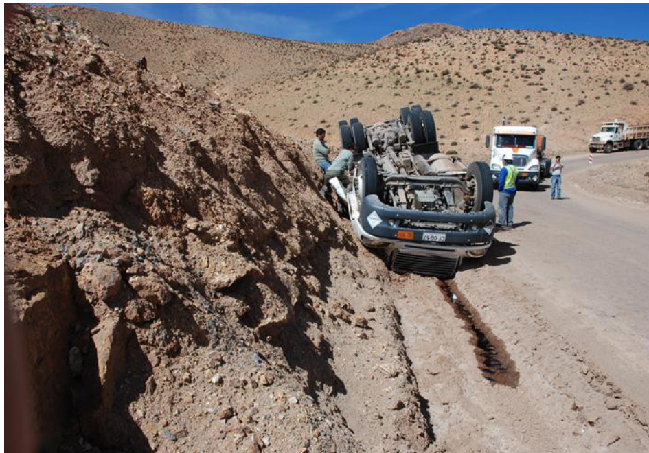
Figure 20 This acid tanker (only the tractor is visible) overturned (a few minutes before the picture) against the uphill slope. Notice that traffic is possible before removal because the road is wide enough. The spill in front is from the fuel tank that did not rupture but started leaking immediately. No acid was spilled (this time) because the tank featured a last generation protected dome.
