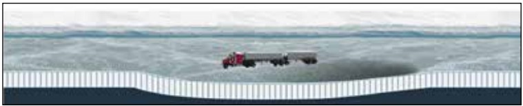
Figure 3.3: A slow moving vehicle causes the ice road to bend and forms a deflection bowl under the vehicle 2
