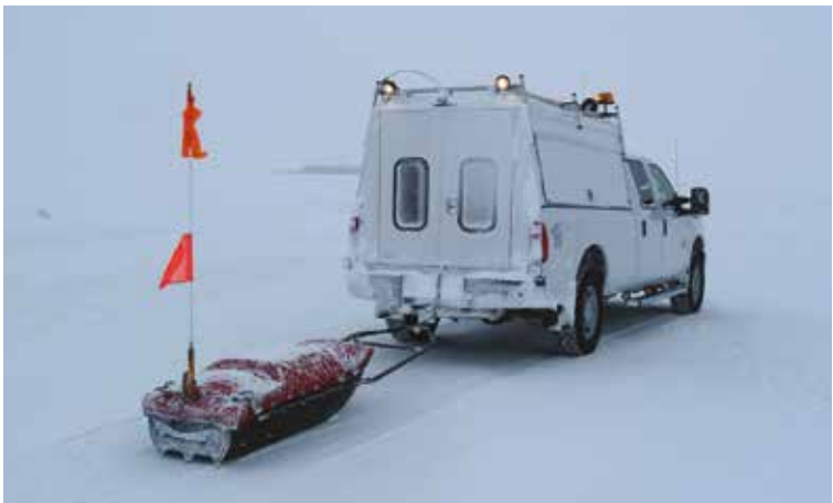
Figure 4.8: Measuring ice thickness with GPR unit.
