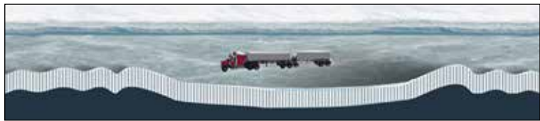
Figure 3.4: A fast moving vehicle causes the ice to bend and creates dynamic waves in the ice ahead and behind the vehicle. 3
