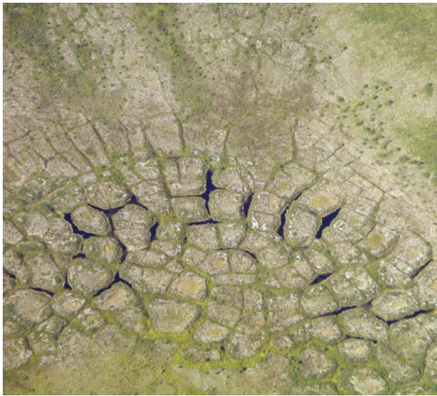
figure 10. In permafrost terrain, avoid road construction on patterned ground.
