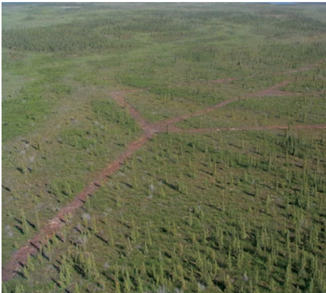
figure 8. Determine if existing roads can be used. Proper planning may have prevented the network of roads shown in this photograph.
