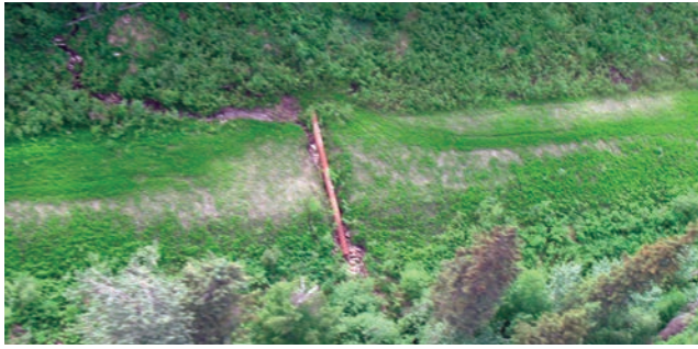
figure 50. This reclaimed site is well contoured and revegetated, but the culvert should be removed.
