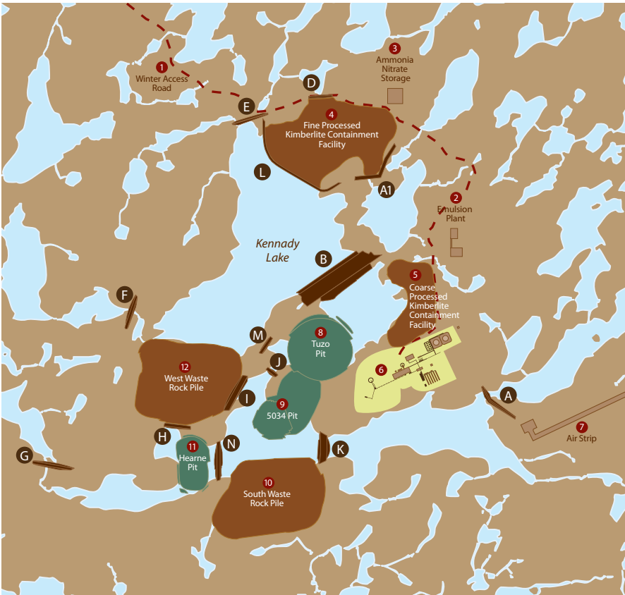
A SERIES OF SMALL DYKES TO BE BUILT AROUND KENNADY LAKE WILL SERVE TWO VERY IMPORTANT PURPOSES. THE FIRST IS TO KEEP CLEAN WATER FROM ENTERING THE MINE SITE. THE SECOND IS TO CONTAIN WATER ON THE MINE SITE UNTIL IT MEETS WATER QUALITY CRITERIA FOR DISCHARGE. THE LAST DYKE - DYKE A - WILL ONLY BE REMOVED WHEN WATER QUALITY IN KENNADY LAKE MEETS WATER QUALITY CRITERIA. DYKES ON THE MAP ARE IDENTIFIED BY A LETTER DESIGNATION.
