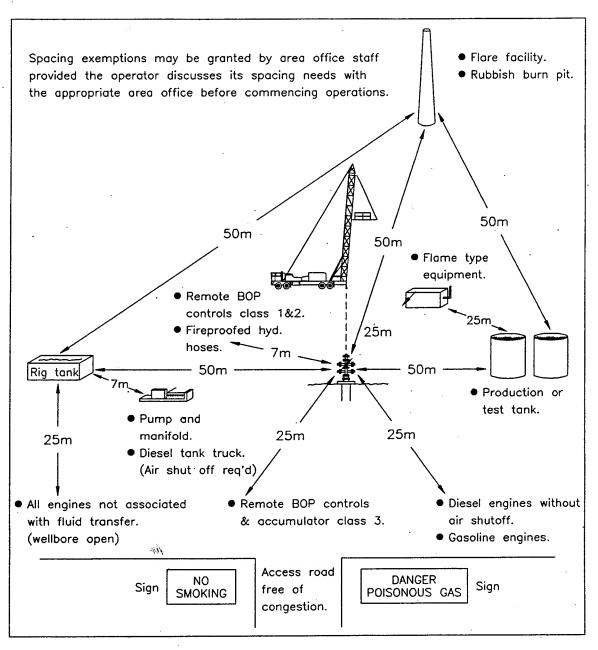
NOTE: The doghouse and light plant must be positioned in accordance with smoking and open flame regulations, and regulations under the Electrical Protection Act.
