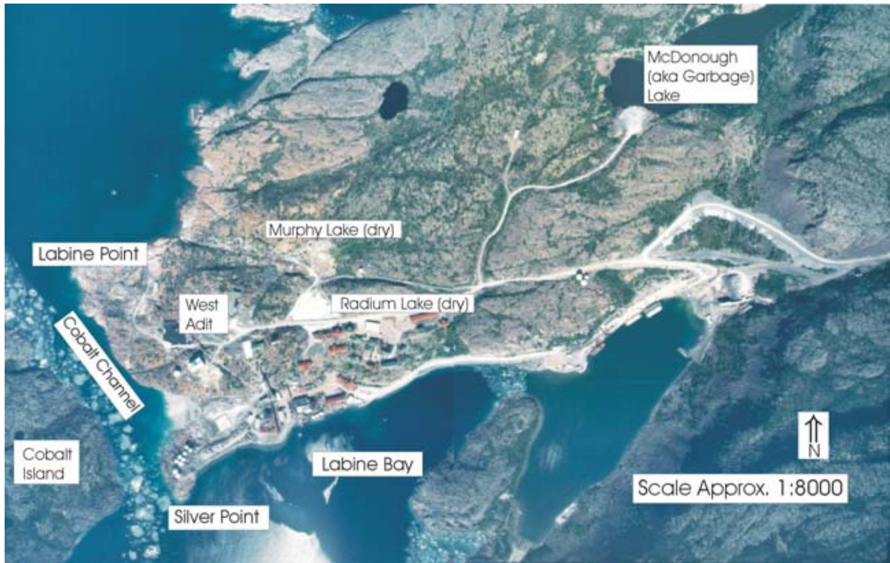
Figure 2.2. Aerial photo (1972) of the Port Radium mine site indicating the tailings deposition areas used during the uranium and silver mining operations
