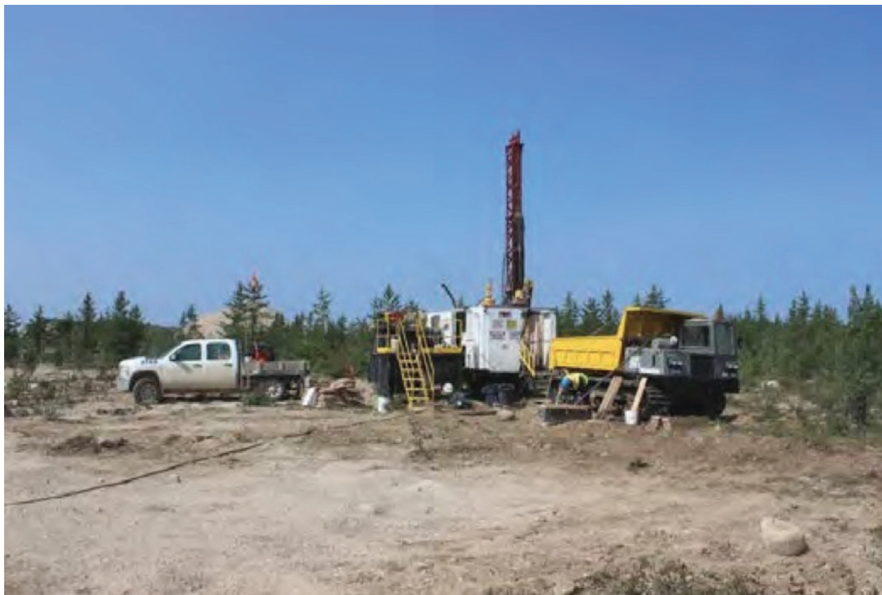
Figure 3: Mineral exploration drilling at Pine Point Mine 2020, photo GNWT Inspection Report
