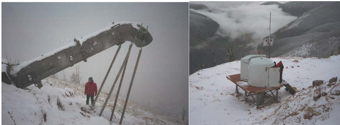
Figure 4-4 – Gas Exploder (left) and Control Shelter (right)
