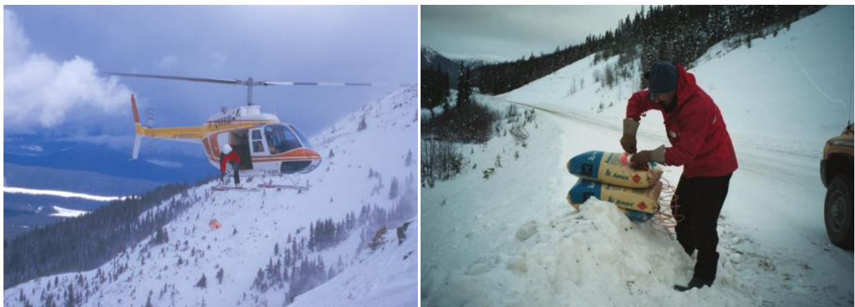
Figure 4-2 - Helicopter Explosive Control and Case Charging
