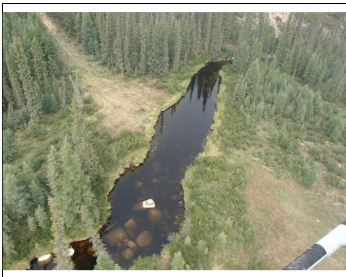
Photo 35: Crossing 14 looking north (downstream); deep pool at crossing with cobbles and gravel substrate, bankfull width = 10 m, bankfull depth = 2.5-3 m (July 2, 2014)
