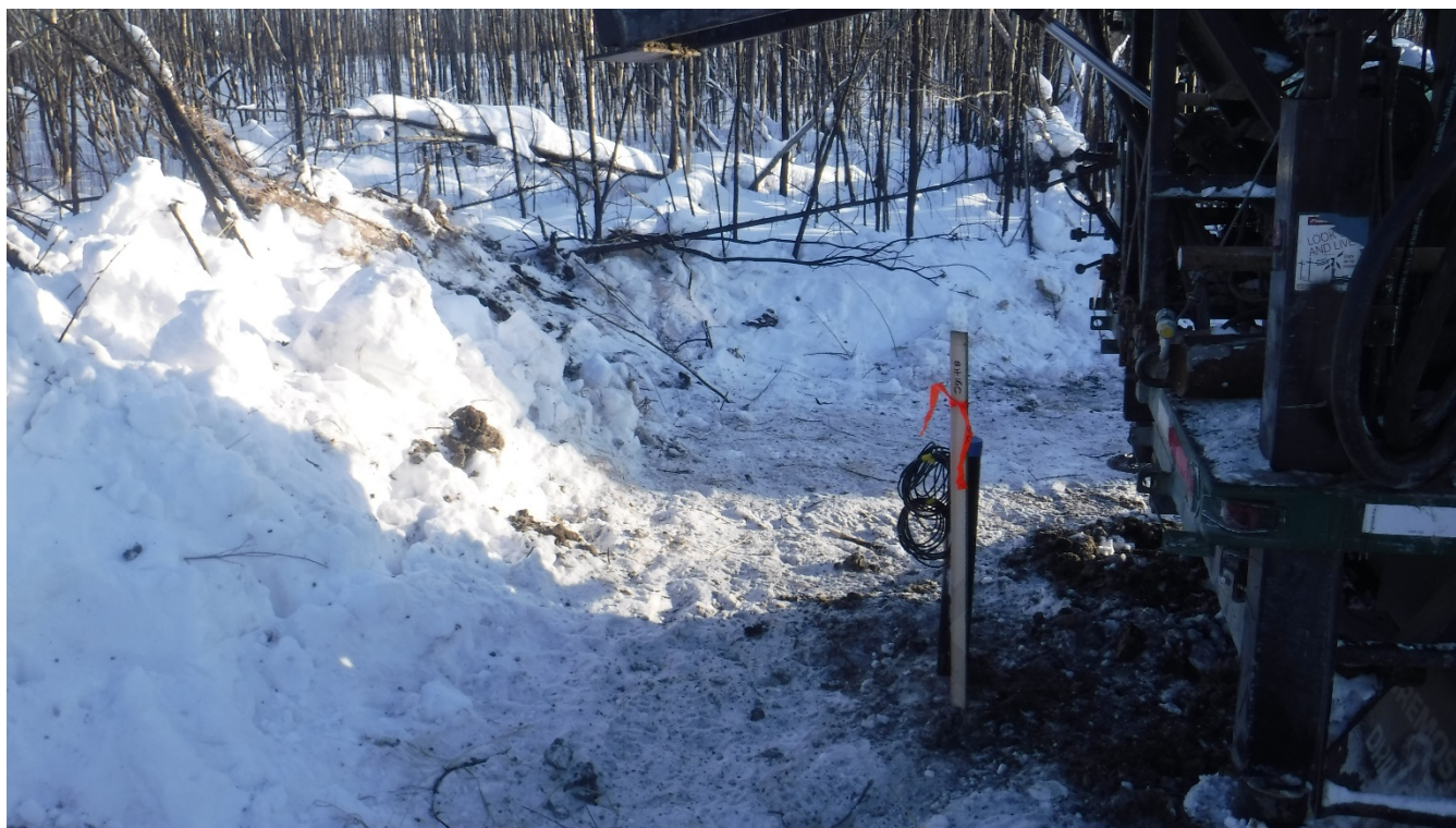
Photo No. 3: Borehole BH17-16C with thermistor cables and PVC pipe.
