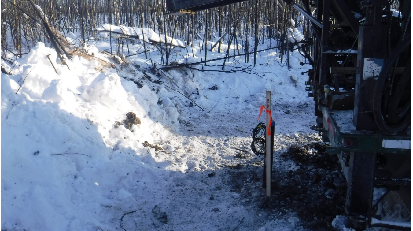
Photo No. 3: Borehole BH17-16C with thermistor cables and PVC pipe.
