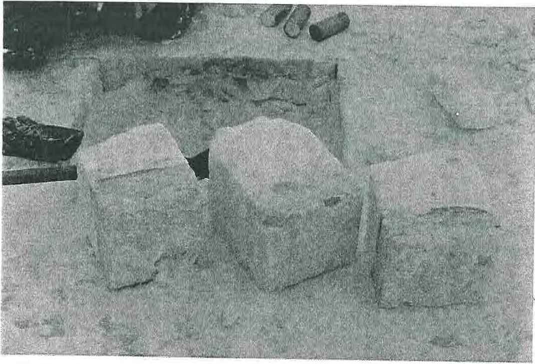
Ice-Capped Snow Roads Are Compacted Snow Roads With Water Applied To The Surface.
