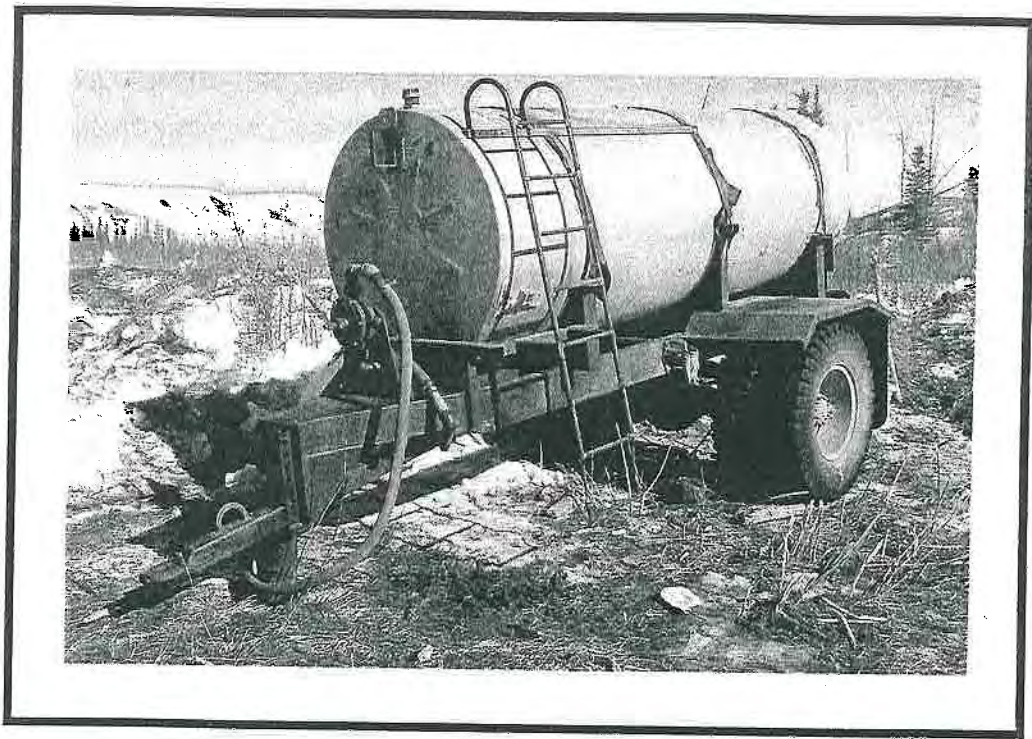
Fuel Storage Should Be On Level Ground, Away From Drainages And Properly Bermed, With Double Valves.
