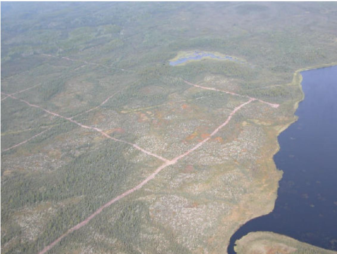
Photo 3. Photo of recent seismic lines in the Cameron Hills. Note "avoidance" cutting of stand of trees in centre right of photo.
