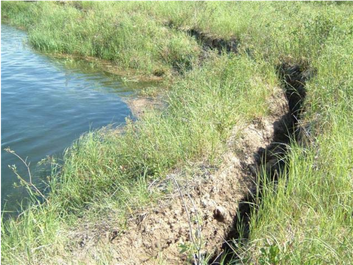
Photo 2.10 Large tension crack at Site 3 (July 9, 2008).
