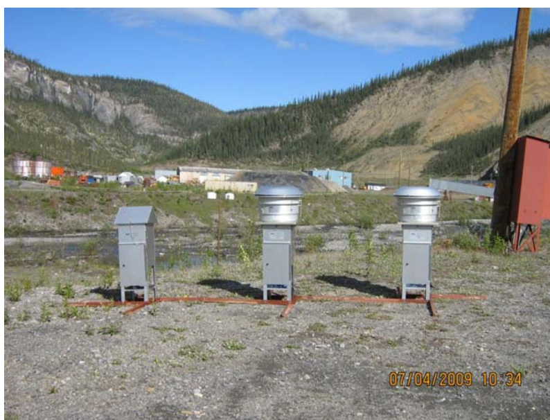
Figure 15: Hi-vol Units Used for Determination of Baseline Concentrations of TSP, PM10 and PM2.5
