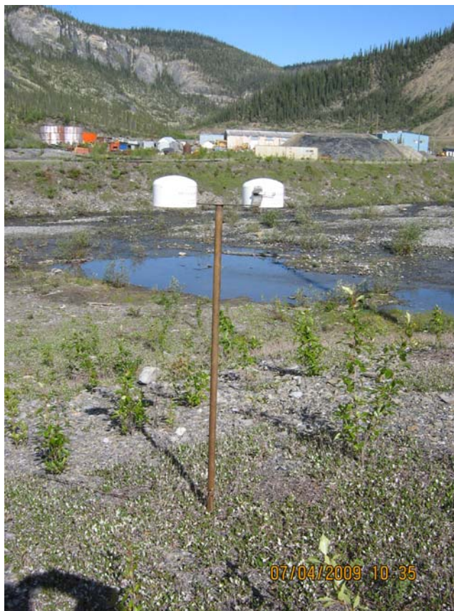
Figure 16: Passive Sampler Units Used for Determination of Baseline Concentrations of NO 2 , SO 2 and O 3
