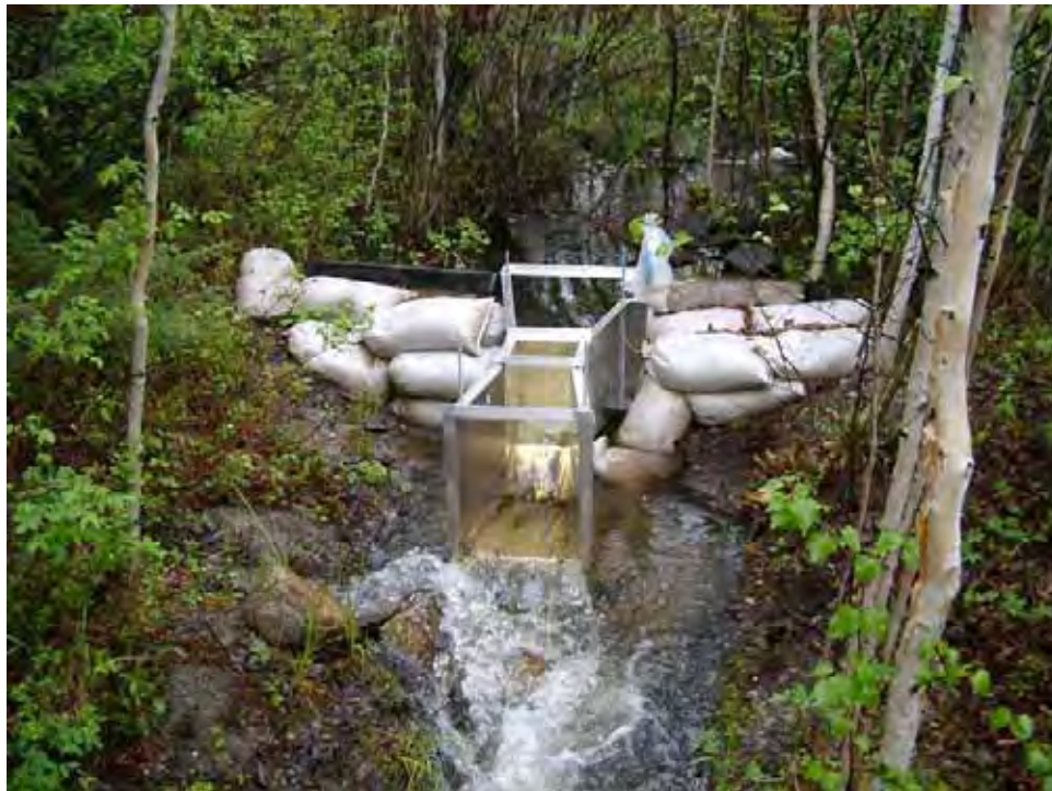
Parshall Flume – Winter Lake Outlet Hydrometric Station (upstream)
