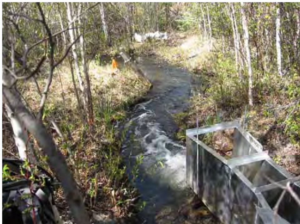
Parshall Flume – Winter Lake Outlet Hydrometric Station (downstream)
