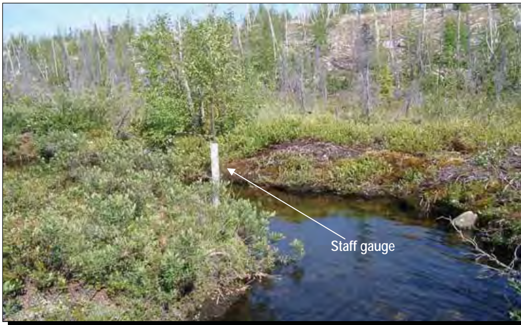
Photo 2 Staff gauge and discharge gauging station
