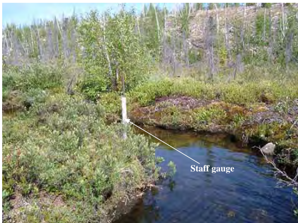
Staff gauge and discharge gauging station
