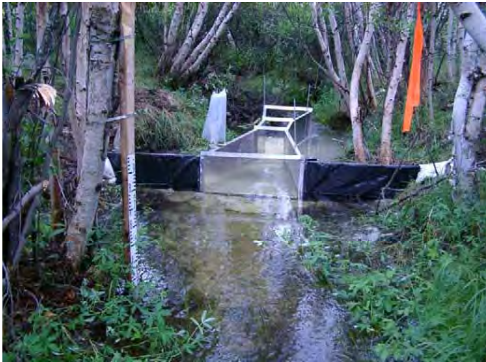
Parshall Flume – Narrow Lake Outlet Hydrometric Station
