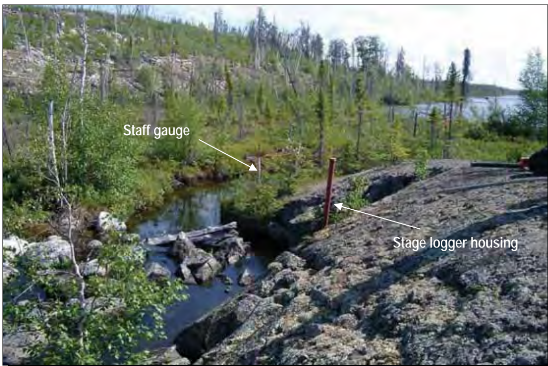
Photo 3 Pressure transducer and data logger
