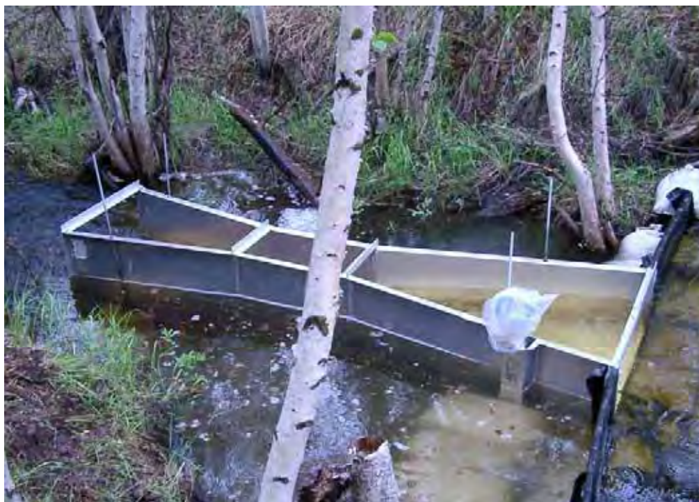
Parshall Flume – Narrow Lake Outlet Hydrometric Station (downstream)
