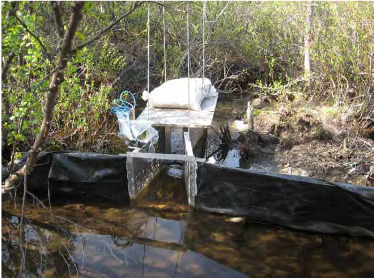
Parshall Flume – Round Lake Outlet Hydrometric Station (downstream)
