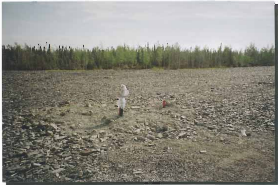
Photo 10 Thermistor and standpipe near center of runway (BH-22) after installation.
