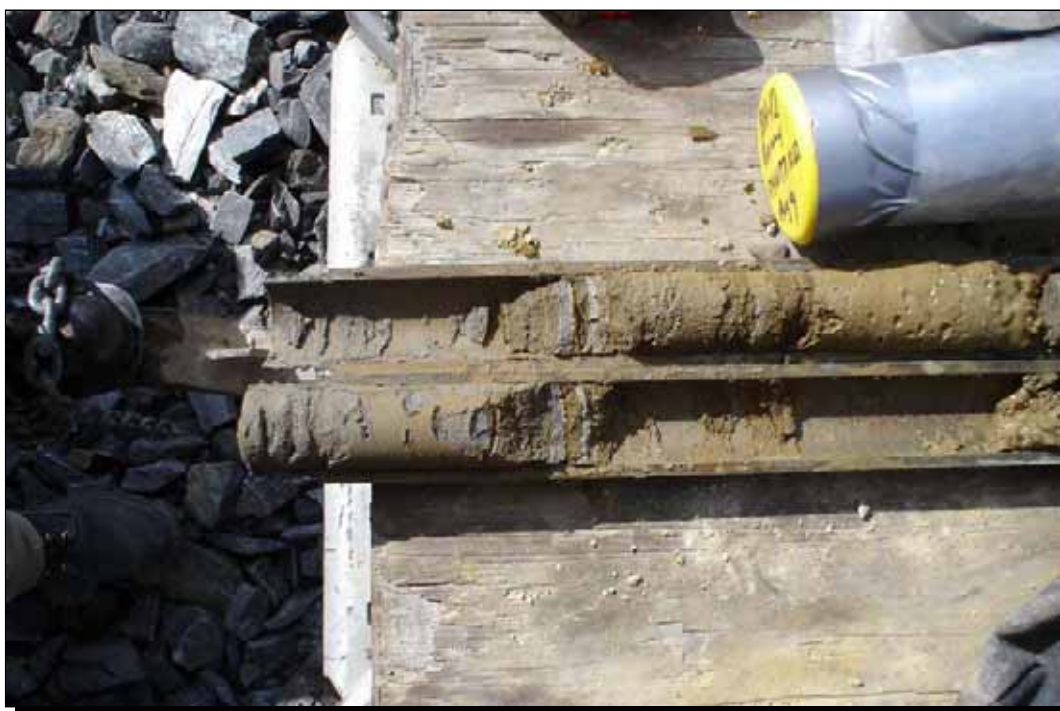
Photo 4 Layers of oxidized and unoxidized tailings in BH-12
