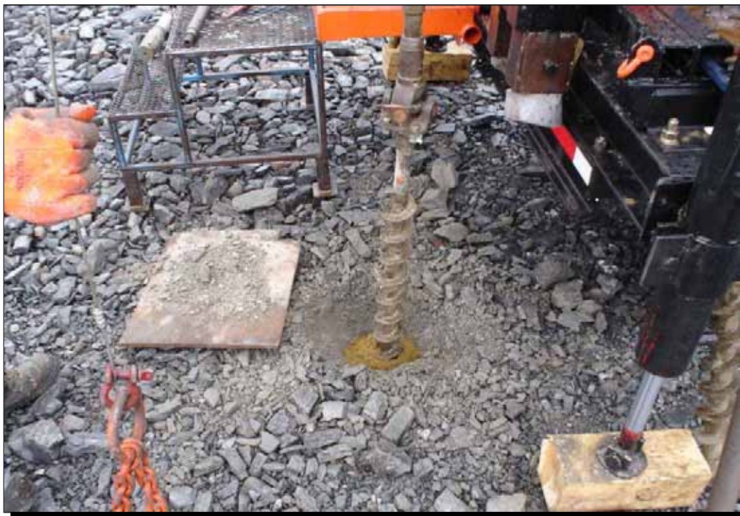
Photo 3 Oxidized tailings coming to the surface during augering of BH-08
