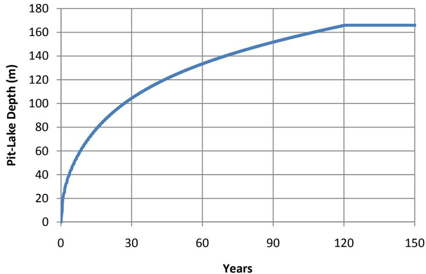
Figure 11.IV.3-1: Flooded Open Pit Filling Results
