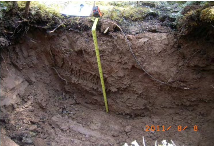
Photo 10: Typical test pit refusal at permafrost.
