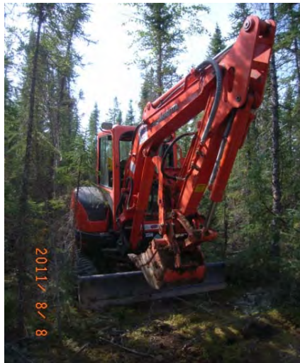
Photo 12: Kubota mini-excavator used for most test pits.
