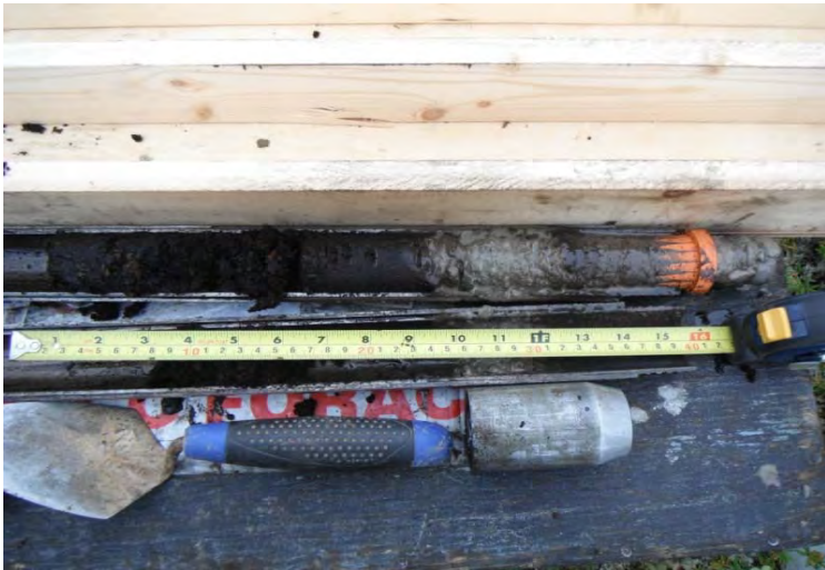
Photo 3: Typical SPT sample in splits.
