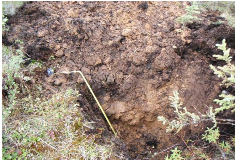
Photo 9: Typical test pit with unstable pit walls.
