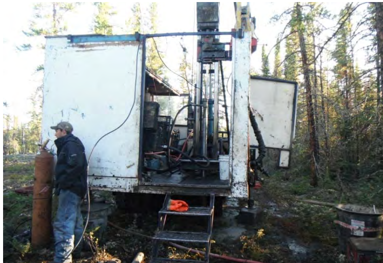
Photo 4: Typical packer test setup.
