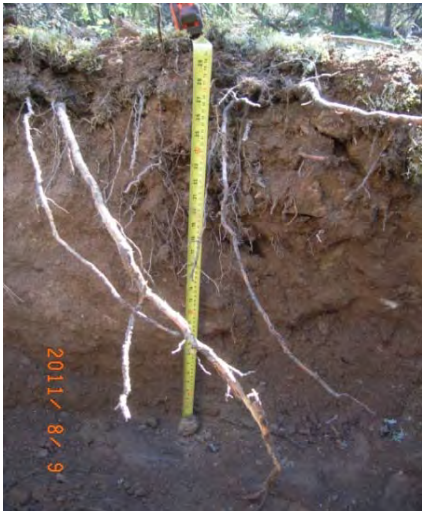
Photo 11: Typical test pit refusal at bedrock.
