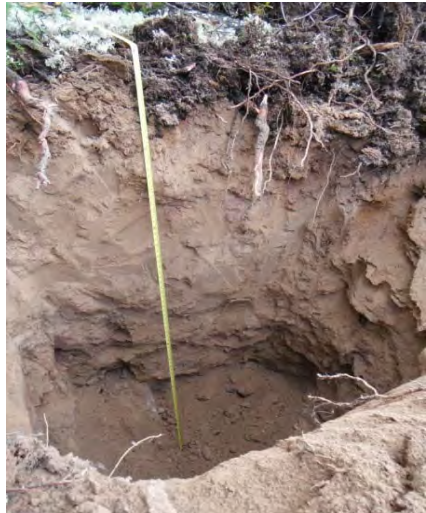
Photo 7: Typical borrow test pit.
