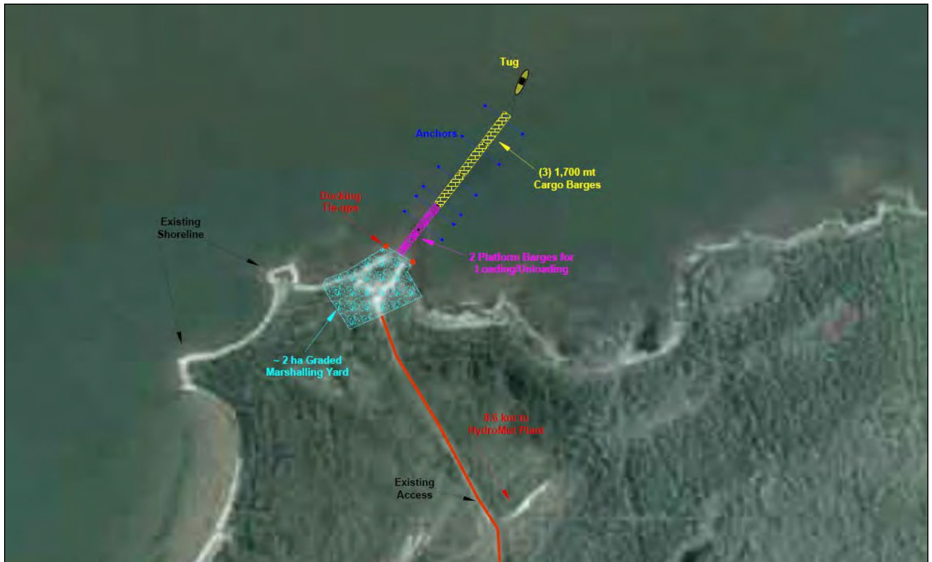
Figure 2.8-8: Hydrometallurgical Plant Site Dock Facility Layout
