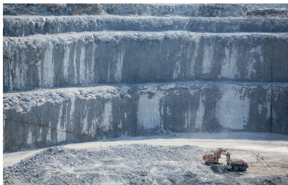
Photo 14: Typical open pit design
