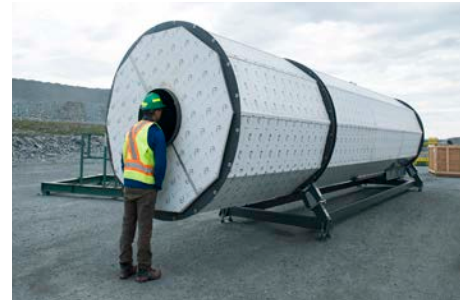
The composter vessel at the Ekati mine
