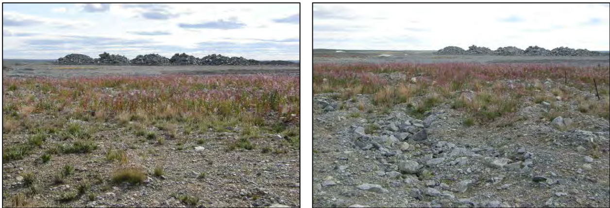
Plate 2.5-2. Topsoil top dressing at the Rock Pad Study with the un-ripped treatment on the left and the deep ripped treatment on the right. August 2014.
