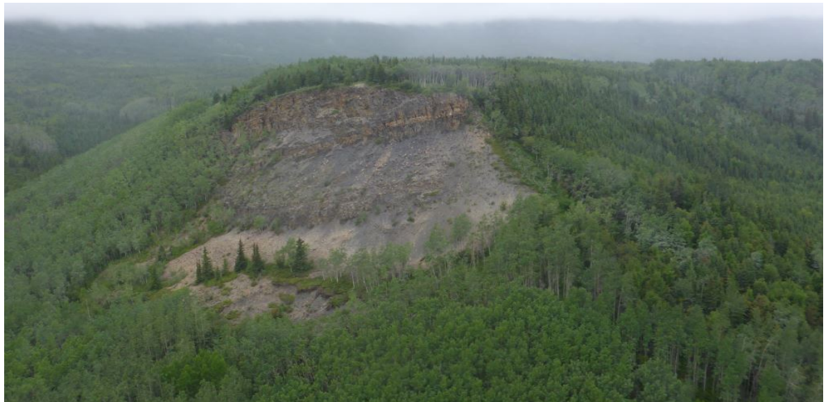
Figure 67. Similar feature found along the section KP 104 to 109, exposed carbonate based cliffs with talus accumulations at the base and expected silt/clay till on the lower slopes suitable for subgrade borrow.
