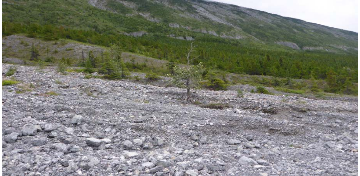
Figure 69. Large source of quality limestone gravels and cobbles available along the proposed alternative route near KP 112. Ideal for crusher operation and a stockpile for future maintenance requirements.
