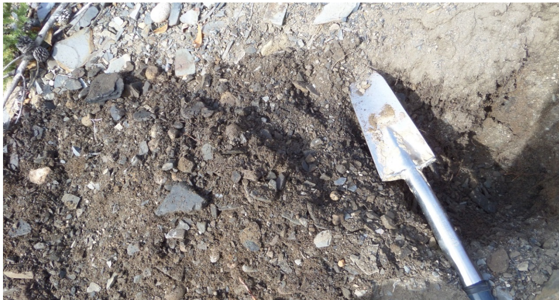
Figure 36: Shale based sandy gravel noted along the old winter road at 59.41 km (BP59)
