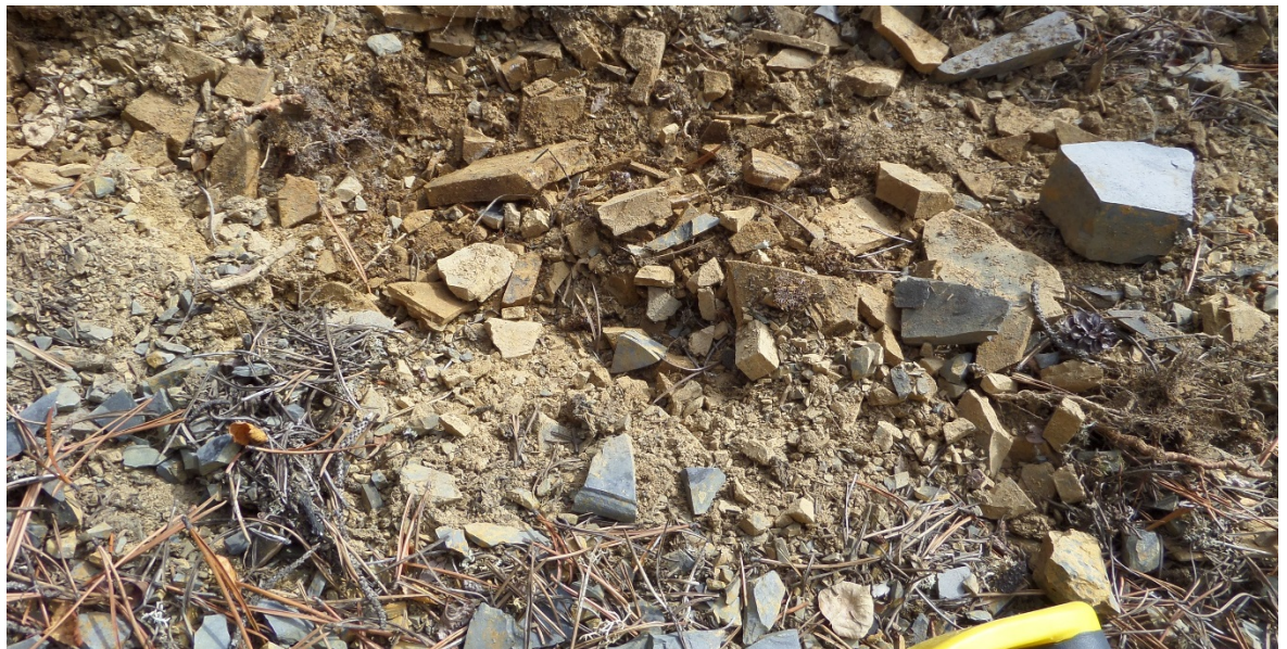
Figure 42: Exposed face with both blocky and fine fissile shale was noted in a rock knob about 200 m southwest of BP65. This material likely extends back close to the road
