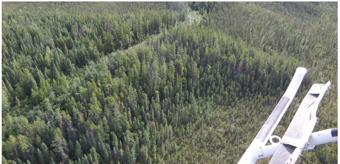
Figure 51: A small ridge of sandy till (BP78) lies under the road route at 78.52 km. The drier material here could be used to construct adjacent overland fills.
