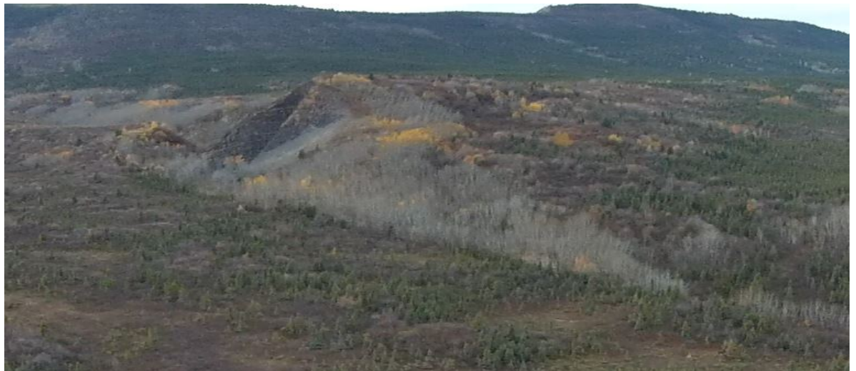
Figure 67: An aerial view of a large, exposed shale rock outcrop a few hundred meters above the proposed road location. It is assumed this rock feature extends down to the road location and could provide an excellent source of blasted/crush surfacing material.
