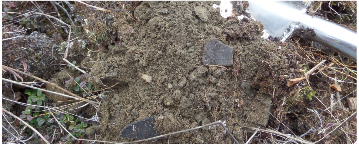
Figure 30: Fine sand with minor gravel and shale showings in the lower bench of BP53.
