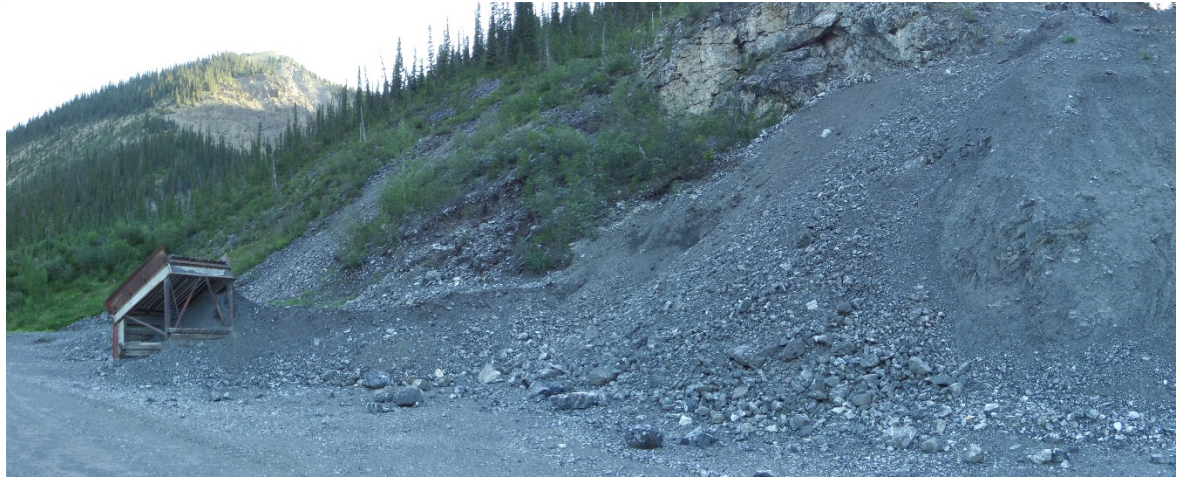
Figure 2: BP2 materials pushed from a higher rock face for screening with a grizzly.
