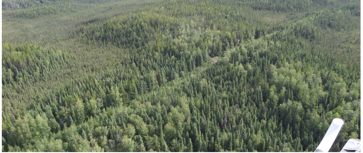
Figure 49: A low ridge of higher sandy till (BP77A) crosses over the road route laterally at 77.22 km. This source of drier material could be used to build some of the overland fills that will be required to cross the wetland.
