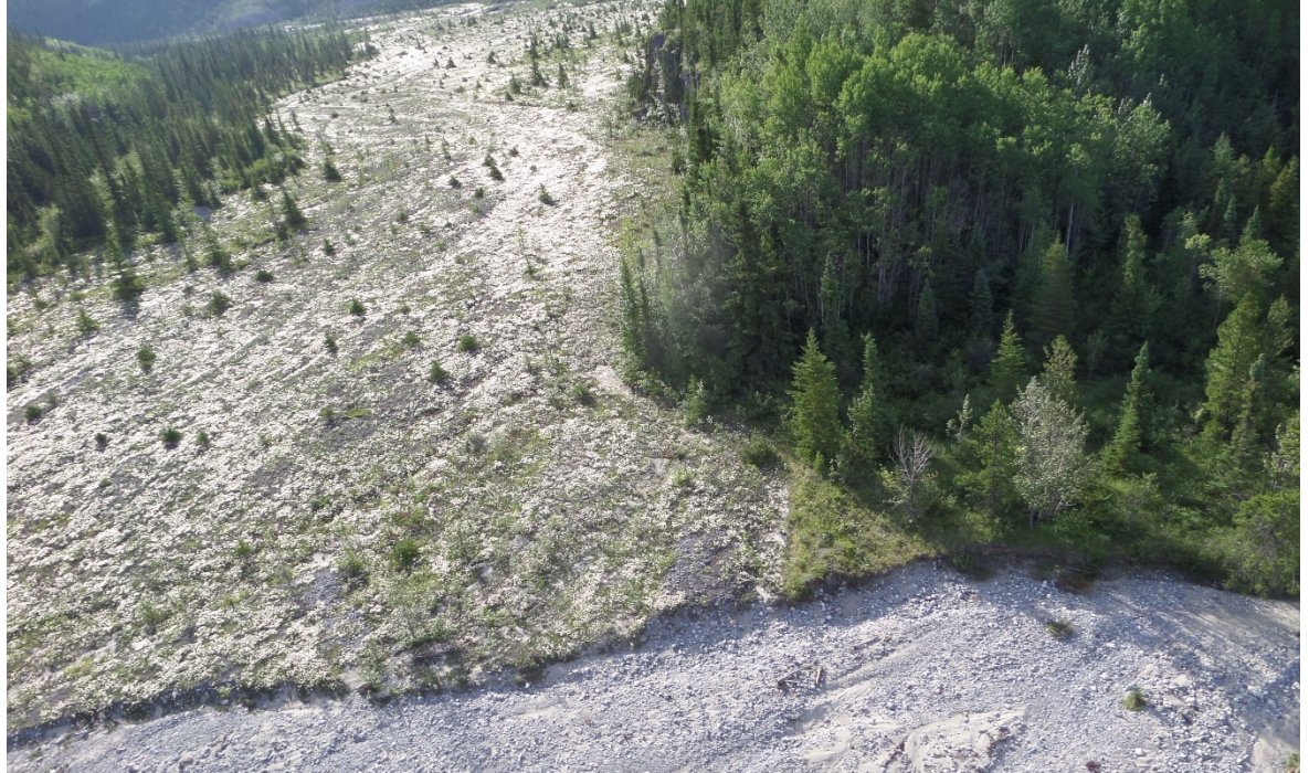
Figure 69: Aerial view (from west) of the dry relict channel left behind when an avulsing streambed changed course at least 35 years ago. The lower part of the photo shows the present day avulsion channel's course, while the upper left side shows the abandoned channel proposed for use by BP123A.
