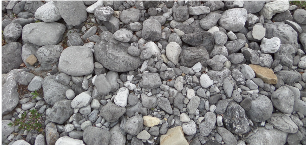
Figure 15: Typical gravel and cobble material available at BP39. This material consists primarily of Paleozoic carbonate rocks as evidenced by the abundance of fossilized coral fragments throughout the aggregates.
