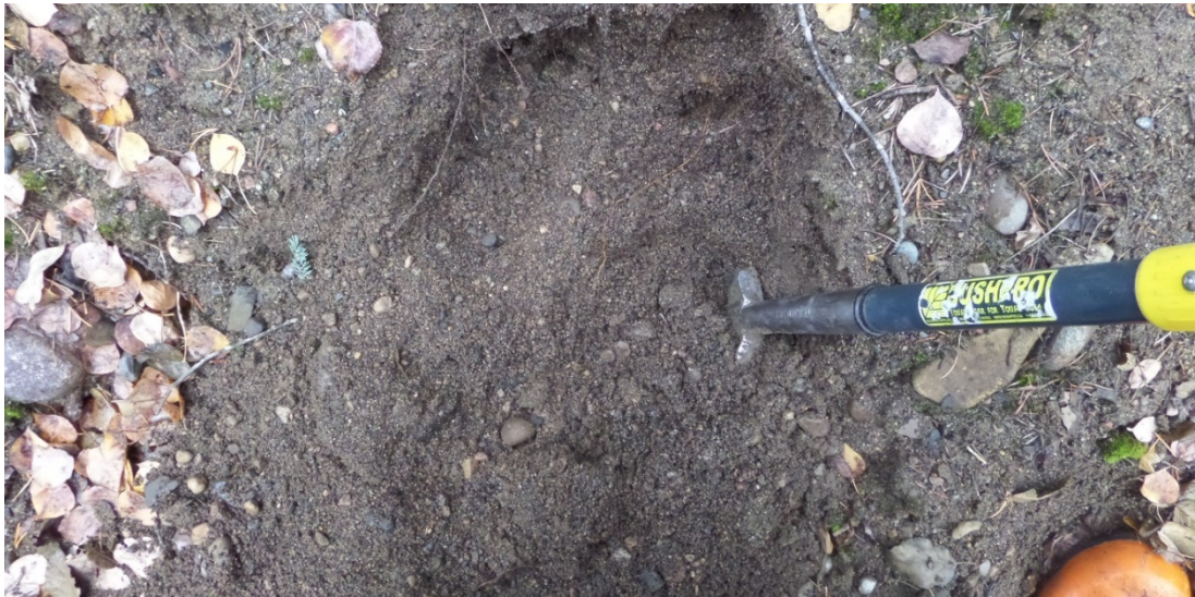
Figure 55: Medium grain sized gravelly sand material found in an existing cut slope at 86.52 km.
