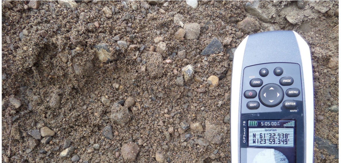
Figure 41: Test pit with well-rounded gravel at BP65. Another test nearby revealed more angular shale gravel content, so the area is somewhat variable for gravel composition.
