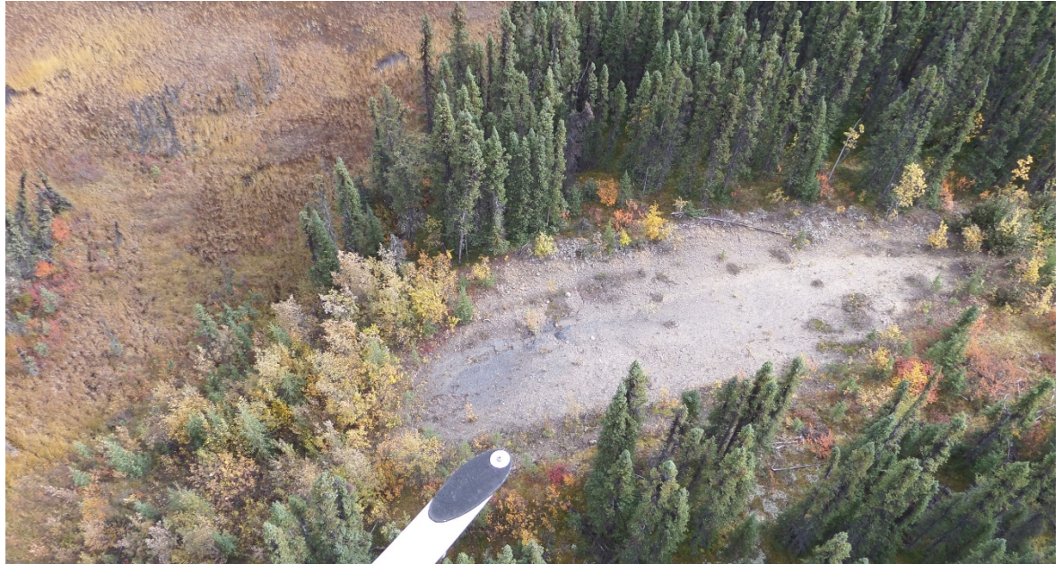
Figure 47: Sandy material in a low hump at 72.86 km (BP72) can be used in a wetland fill.
