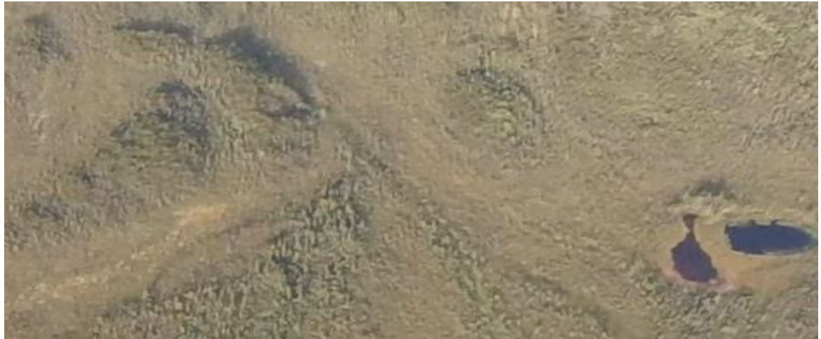
Figure 59: Aerial view of the landscape from KP 90 to 95. Patches/islands of dry, esker type terrain covered with lodgepole pine/aspen. These humps will provide borrow material to overland the lower, depressed permafrost (likely ice-rich) sections in between.
