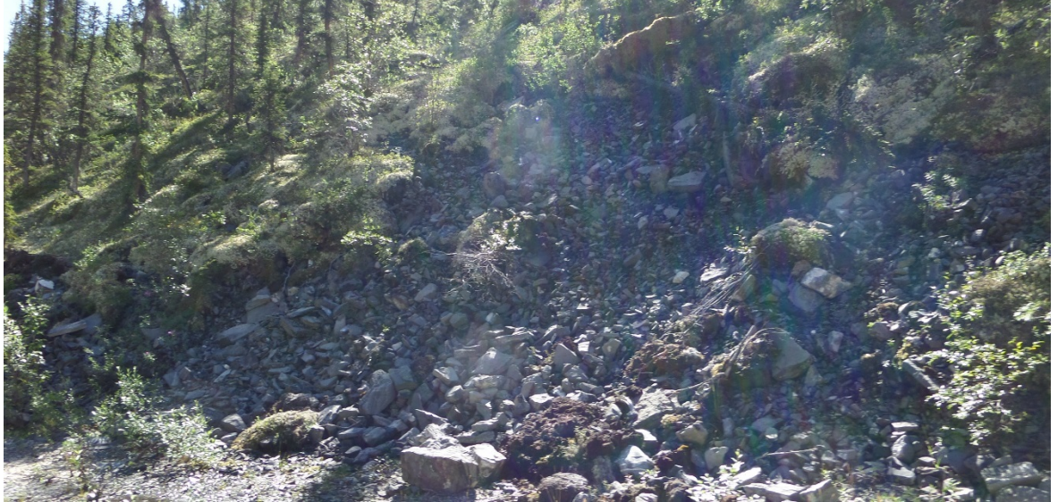
Figure 8: BP10 material showing a wide size gradation. Also note some evidence of creep along the slope – this is assumed to be related to permafrost.
