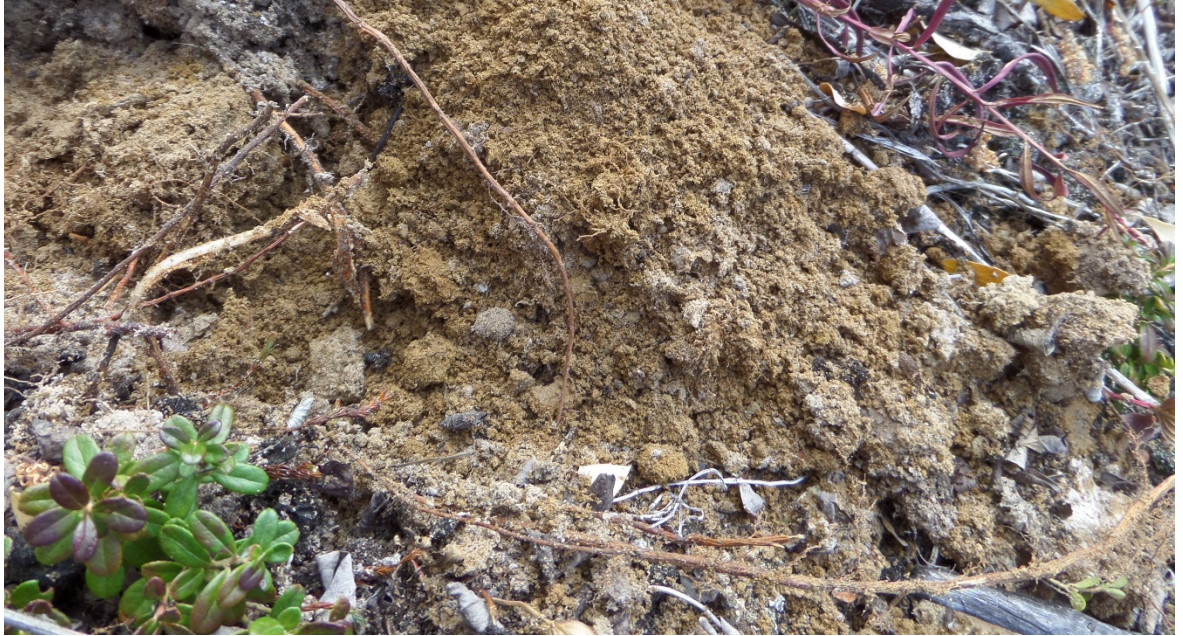
Figure 28: The fine sand in BP51 is a potential overland subgrade borrow source on the west side of a section of deep organic lowland running from 51.75 km to 52.95 km.
