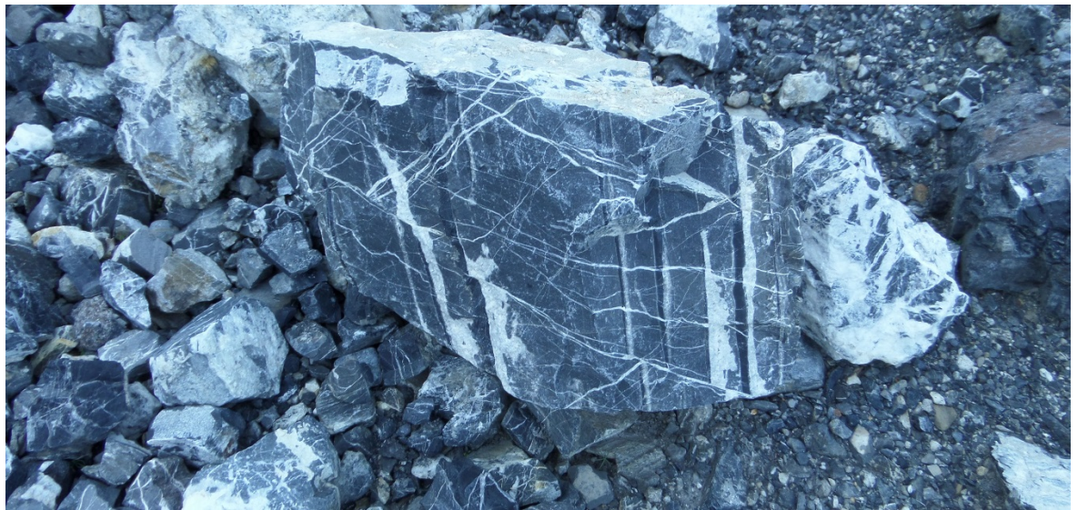
Figure 3: Close up of the BP2 mudstone with sparry calcite cementing.
