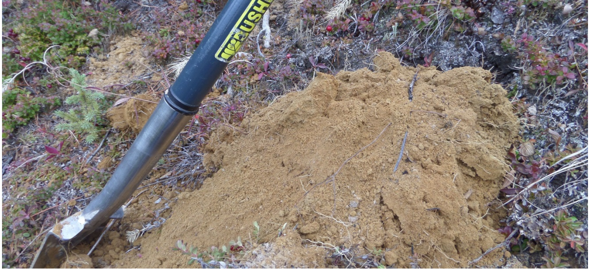
Figure 27: The fine sand in BP50 is potential fill for crossing over nearby lowlands.
