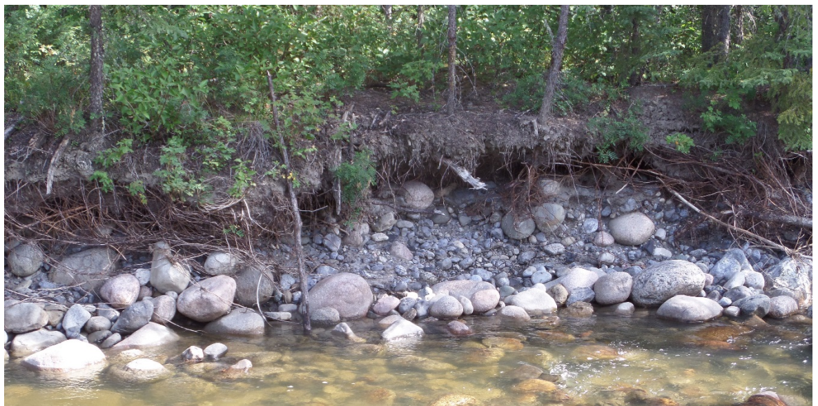
Figure 58: View of some of the material deposited within the existing river bank to the west of the proposed BP87 location. This material is assumed to be typical of the deposition in the borrow area and it would need to be crushed for road surfacing.
