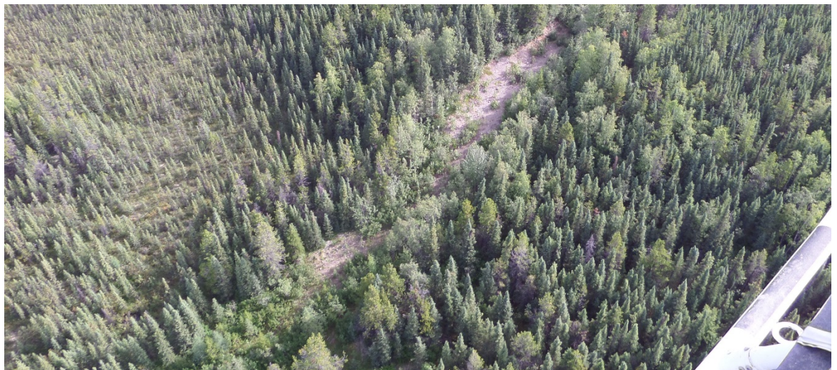
Figure 48: Another small sand hump at 76.23 km can provide fill for a wetland crossing.
