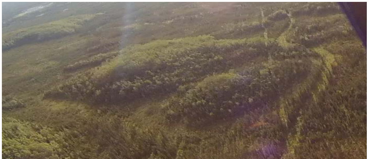
Figure 62: Dry elevated “humps” covered with lodgepole pine and aspen should provide adequate silty sand type material for overland sections, particularly in the proposed switchback section KP 97 to 102.
