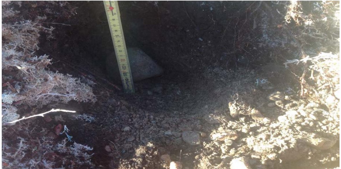
Figure 12: Large esker like deposit of glacial-fluvial gravel at 15.8 km.
