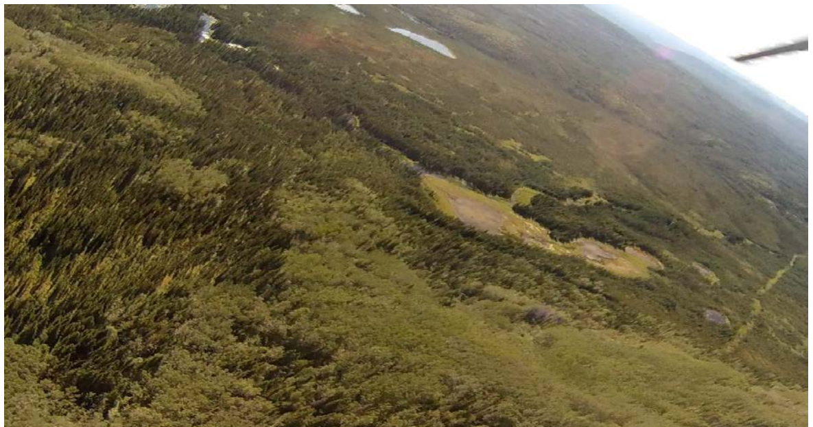
Figure 60: Aerial view of the landscape near KP 96. Borrow to be extracted from elevated dry humps covered mainly with aspen and lodgepole pine.
