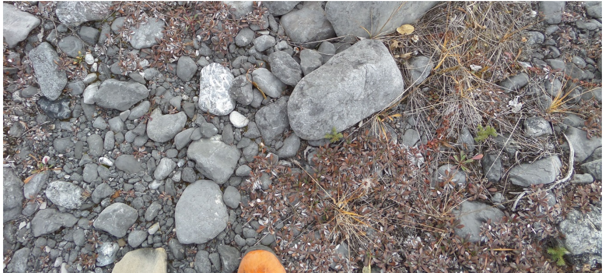
Figure 24: Typical BP47B alluvial deposit materials derived from carbonate parent rock.
