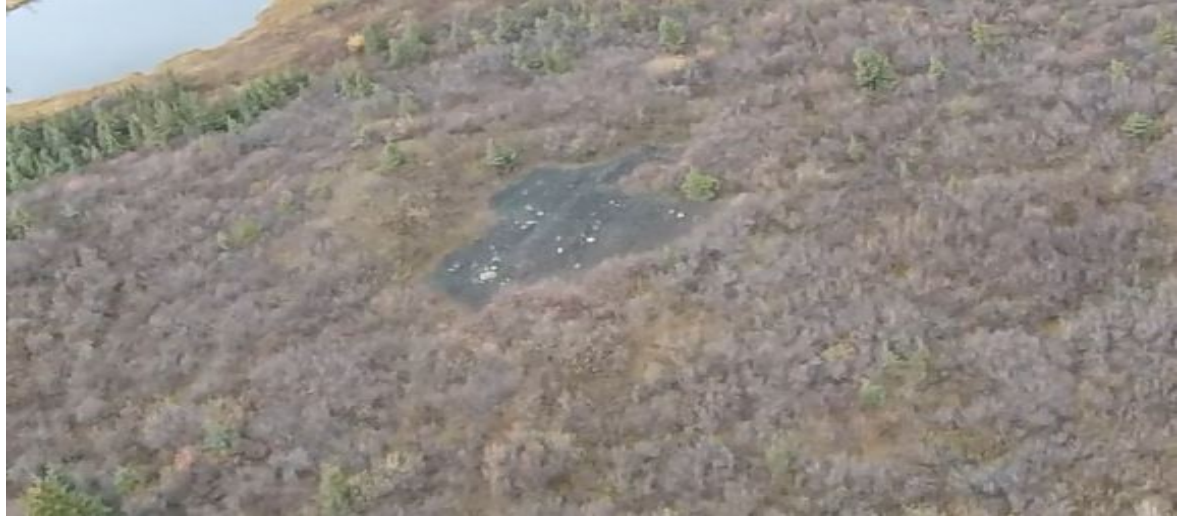
Figure 68: A low level fly over identified this potential shale rock deposit. The proposed road is located through this feature.
