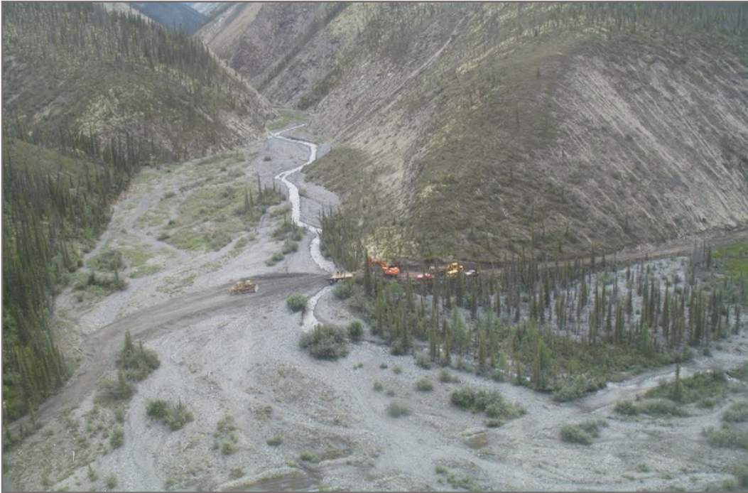
Photo 1: KP 6.1, Casket Creek. Aerial image viewing upstream, 2008. Active alluvial fan area with split flows and shifting of the main channel being likely during major flood events.
