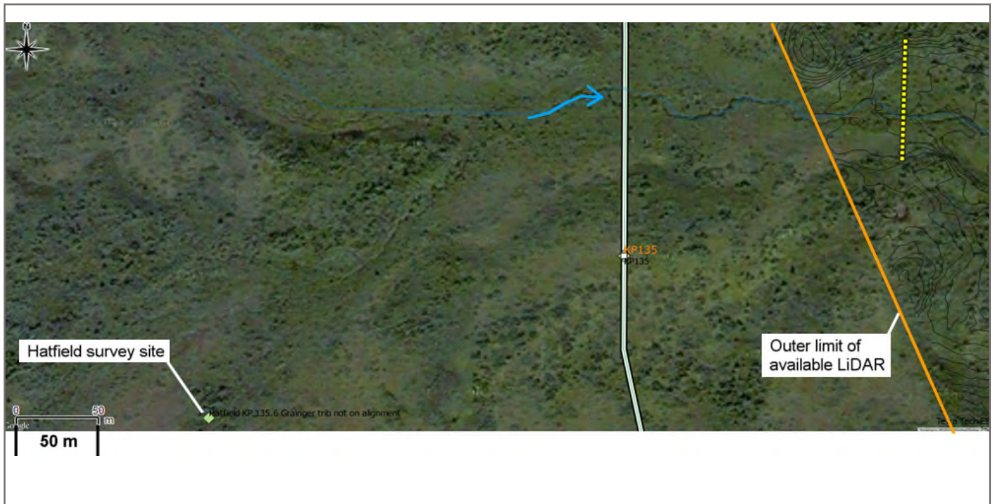
Figure 34: KP 134.9 Grainger Trib. (Hatfield KP 135.6). 2014 road alignment shown on Google Earth image. Flow is left to right. 2012 LiDAR data and orthophoto imagery not available for the 2014 crossing location due to alignment change. Channel cross section view taken at yellow dashed line viewing downstream, and located downstream from road crossing in reach with available LiDAR data.
