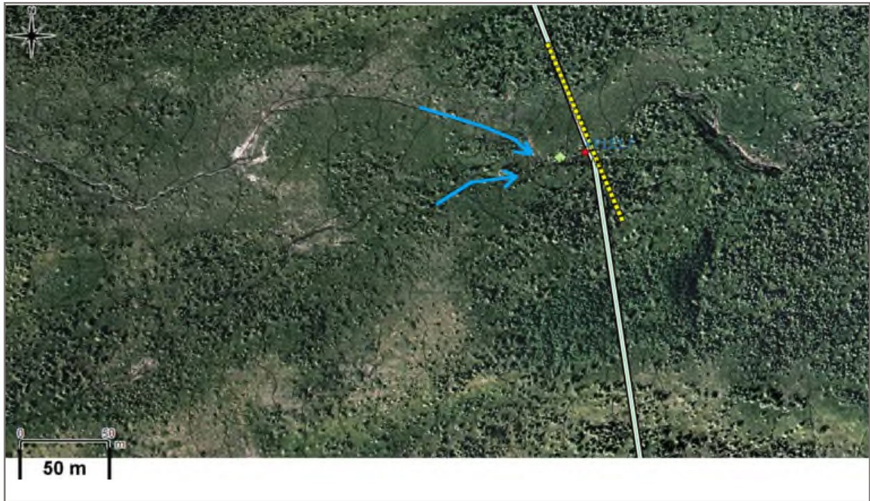
Figure 32: KP 133.2 Grainger Trib. (Hatfield KP 133.7). 2014 road alignment shown on 2012 orthophoto image. Flow is left to right. Channel cross section view taken at yellow dashed line viewing downstream.
