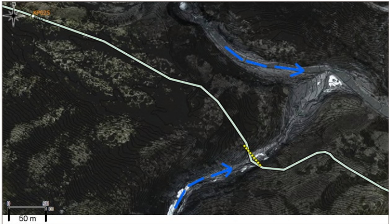
Figure 6: KP 25.3, Sundog Tributary. 2014 road alignment shown on 2012 orthophoto image. Flow is left to right. Channel cross section view taken at yellow dashed line viewing downstream.
