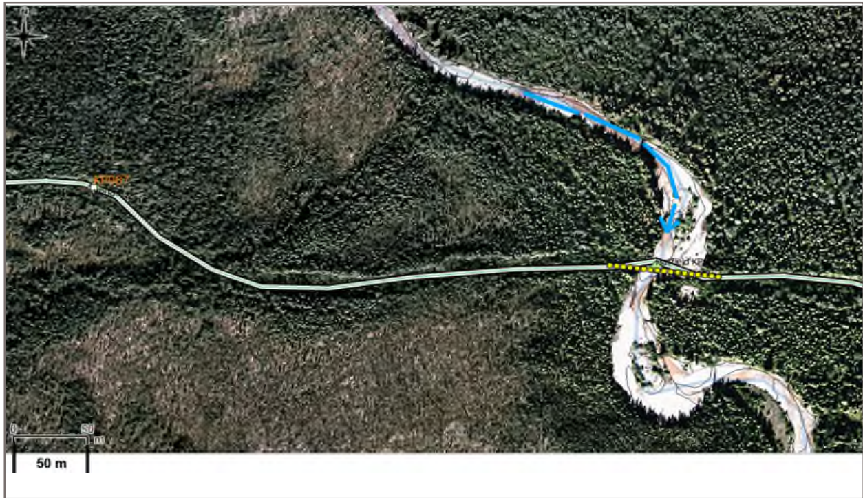
Figure 20: KP 87.4 Tetcela Trib at Old Road. 2014 road alignment shown on 2012 orthophoto image. Flow is top to bottom. Channel cross section view taken at yellow dashed line viewing downstream.
