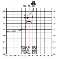
Cross section example: 7 m "vertical fall" and high cut in rock at km 36.9. Implementation of berms/barriers downhill-side, gabions uphill-side seems difficult due to the lack of space.
