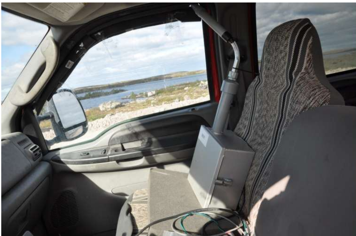
Figure 5: E-Sampler with TSP Inlet Head Mounted on Pick-Up Truck
