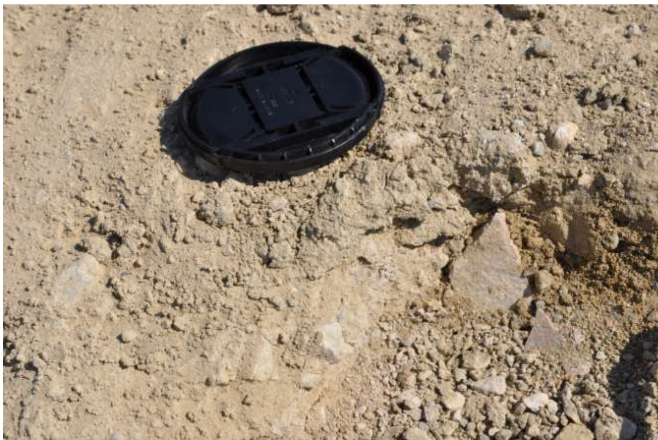
Figure 18: Victor Mine Road Limestone Material with Fine Grained, Cemented Character (Photo: A. Pickup, 2011)
