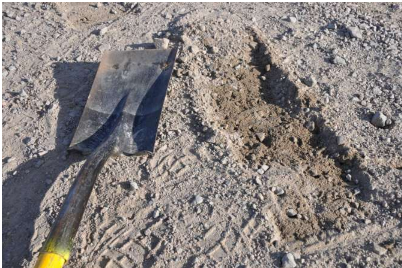
Figure 20: Snap Lake Road Granitic Material Showing Pulverized Material and Depth of Moisture Retention below Surface (Photo: A. Pickup 2011)
