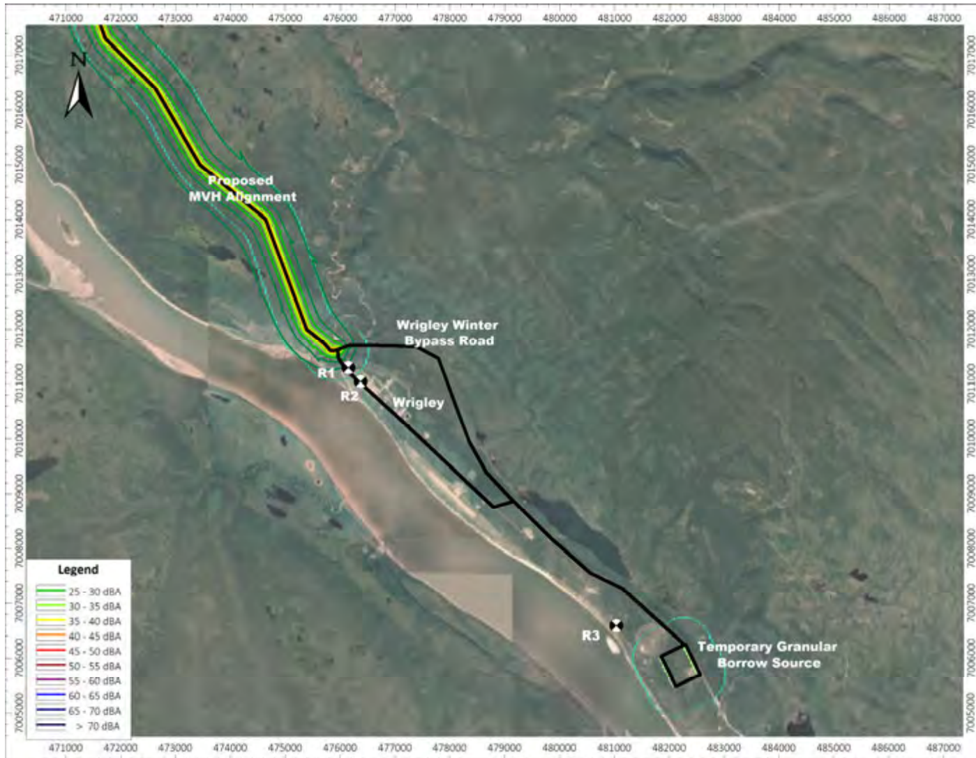
Figure 13B.4 Noise Map - Operations and Maintenance Phase - Traffic Noise ( L_{eq-24hr} )
