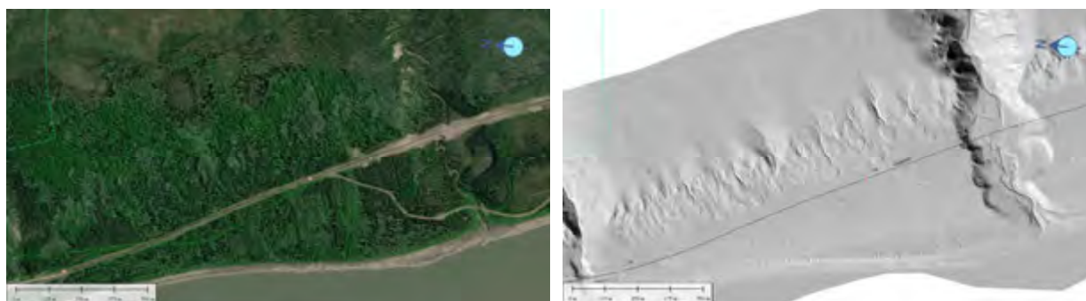
Landslides upslope from the MVH alignment near Vermillion Creek South (MVH KM 752 to KM 754)
